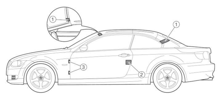
1. The areas mark the zones at which the roof can be cut off:
