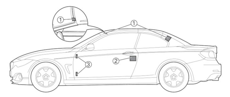
1. The areas mark the zones at which the roof can be cut off:
