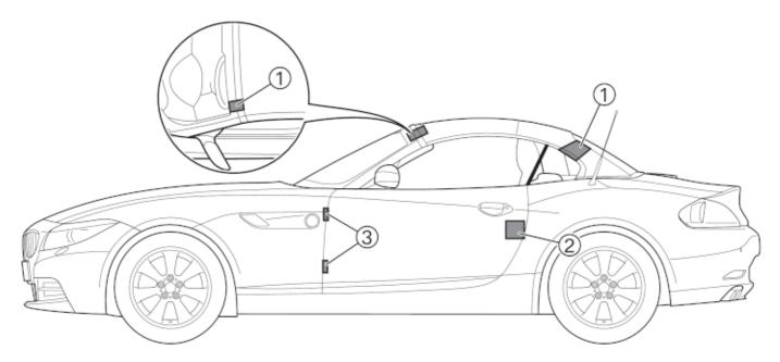
1. The areas mark the zones at which the roof can be cut off:
