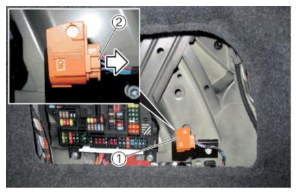
Unlock connector (1) for high-voltage emergency separation point (2) and pull apart in direction of arrow.
