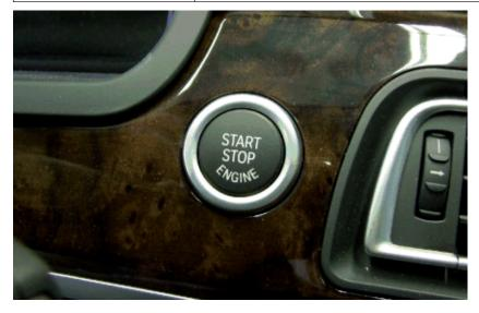
With the engine running or with the displays in the instrument cluster being activated, push button "START STOP ENGINE" to switch off ignition.
