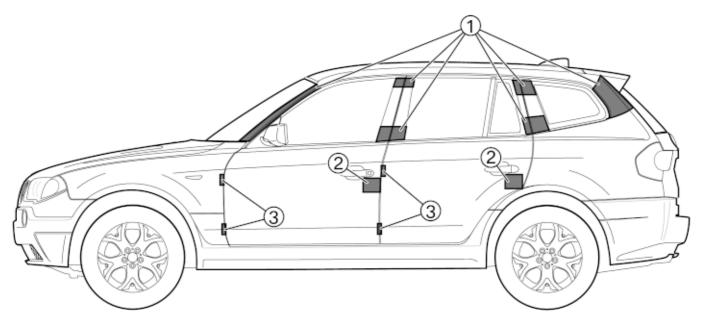
The areas mark the zones at which the roof can be cut off. Modern heavy duty cutting equipment is mandatory for cutting the body. Older hydraulic cutting tools could be overloaded.
