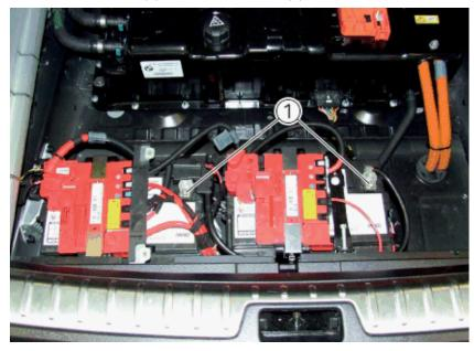
Loosen the nuts (1) and pull the battery earth leads out toward the top. Cover negative battery terminal in order to rule out contact with battery earth lead.
