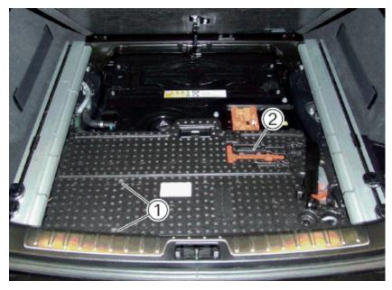
Release the screws (1) with a screwdriver (2) and remove the cover.
